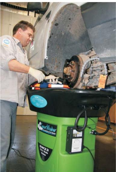
Curtis Thurman, equipment repair technician, uses a SmartWasher® to clean brake and rotor assembly instead of using harmful solvents.
